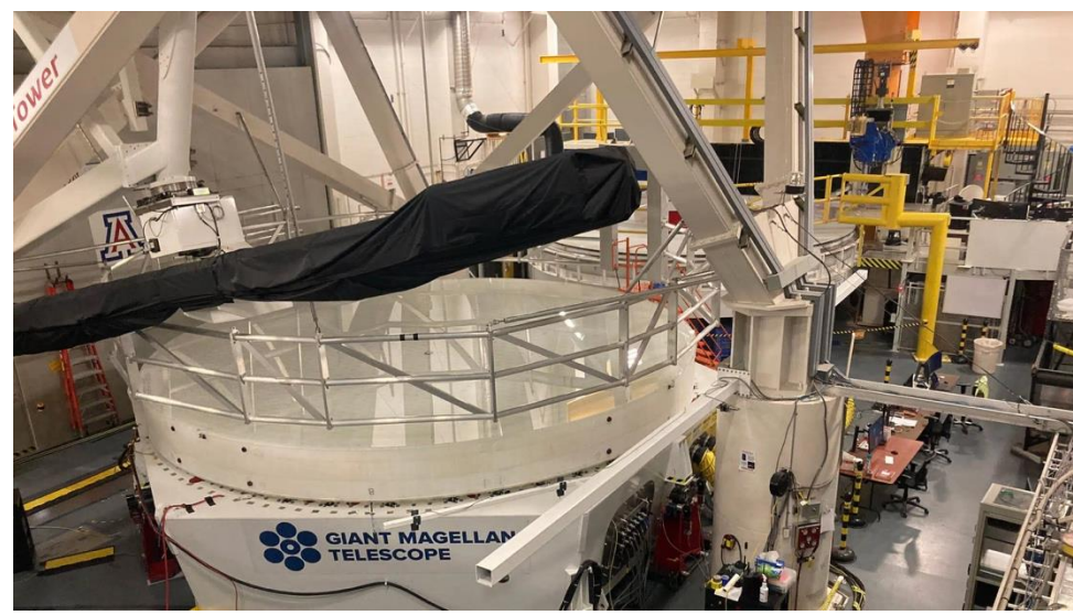
Supporting system prototype integrated with a 8.4-meter mirror (Credit: GMTO)
